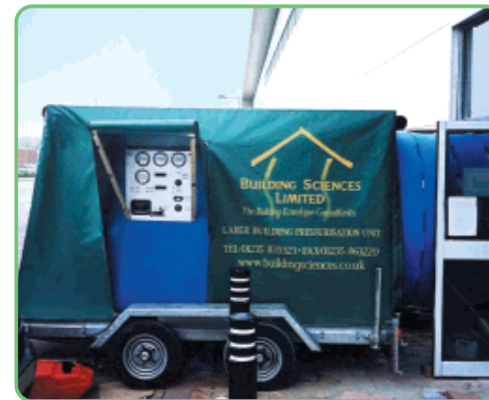
Figure 4. Large building air pressurisation testing equipment
