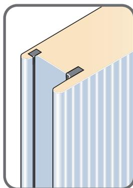
Internal: Simpler typical T&G Joint
